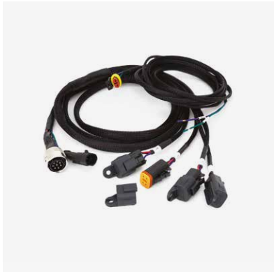
FOUR-LAMP WIRING KIT (CARBON-6) 4L-CS-185 Includes ITT cannon connector. 1.85m lamp cables. Additional wires for Fog/E-mark modes.
