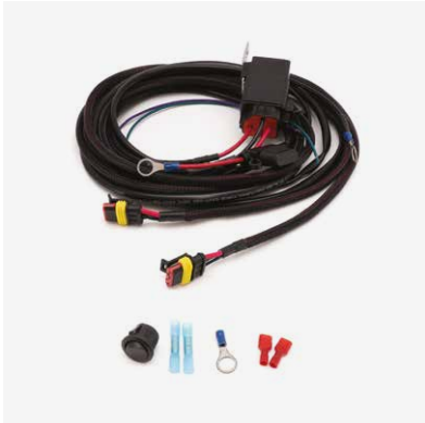
TWO-LAMP WIRING KIT (POSITION LIGHT) 1L-LP-PL-120 3-pin superseal connectors. 1.2m cable length. 12v relay. 30A fuse.
