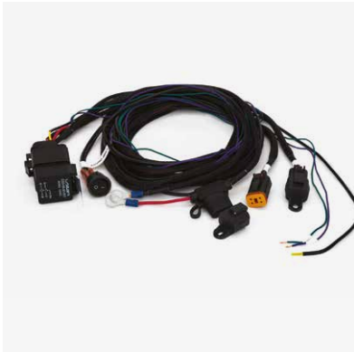
TWO-LAMP WIRING KIT (CARBON-6) 2L-DT4-235 4-pin Deutsch connectors. 2.35m cable lengths. 12v relay. 25A fuse.
