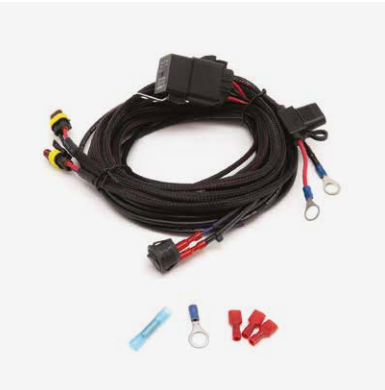
TWO-LAMP WIRING KIT (LOW POWER) 2L-LP-120 2-pin superseal connectors. 1.2m cable length. 12v relay. 35A fuse.
